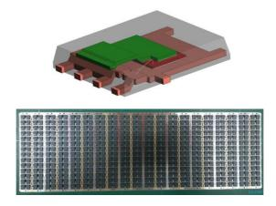
UTAC Holdings Ltd. (UTAC), a global semiconductor test and assembly services provider, is announcing a punch copper (Cu) clip packaging solution for power MOSFET market.
